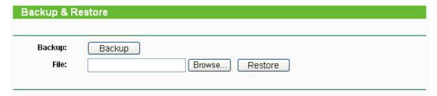
Figure 5-30 Save or Restore the Configuration
