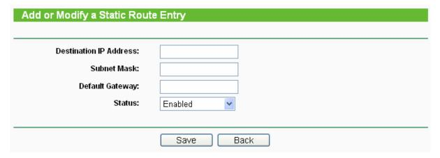
Figure 4-45 Add or Modify a Static Route Entry
