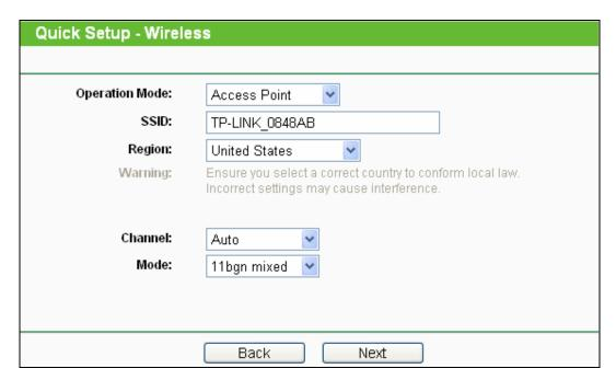
Figure 3-13 Quick Setup - Access Point Mode
