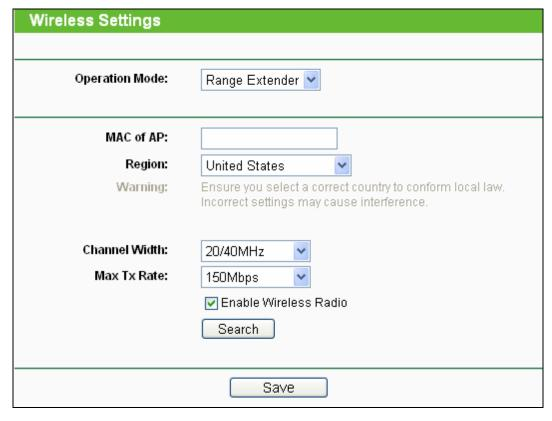
Figure 4-8 Wireless Settings in Range Extender mode
